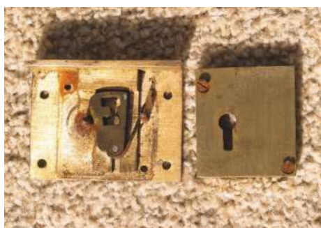
A George IV lock with cover plate removed to show levers and spring
